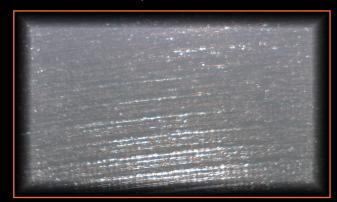
Stamped aluminum membrane under a microscope.
